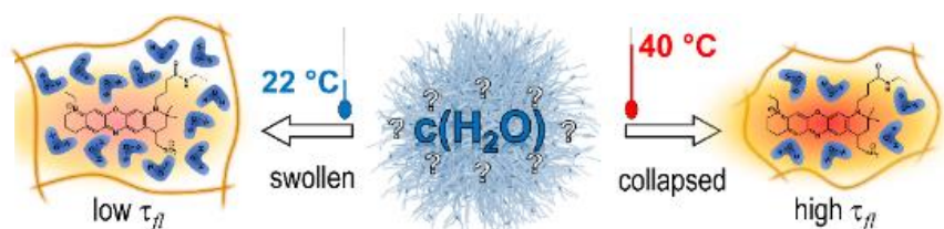
Scheme 1: Estimation of water content in ATTO 655-labelled microgels in their swollen and collapsed state by measuring \tau_{fl} .
