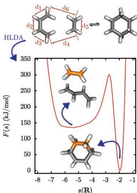
**Fig. 5:** Free energy profile for the Diels-Alder reaction of 1,3-butadiene with ethene as a function of the HLDA CV obtained using the set of six bond distances as basis descriptor.
