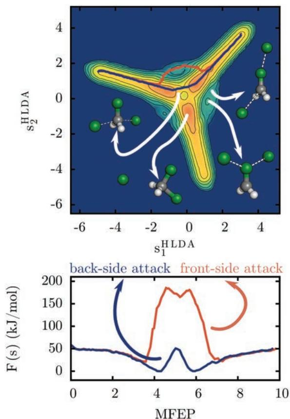
**Fig. 8:** Upper panel: free energy surface for the nucleophilic substitution of a chlorine atom in dichloromethane showing the two possible reaction paths and associated relevant reference structures. Lower panel: minimum free energy paths along for the two possible mechanisms of the reaction, namely the low-barrier back-side attack (blue line), and the high-barrier front-side attack (orange line).
